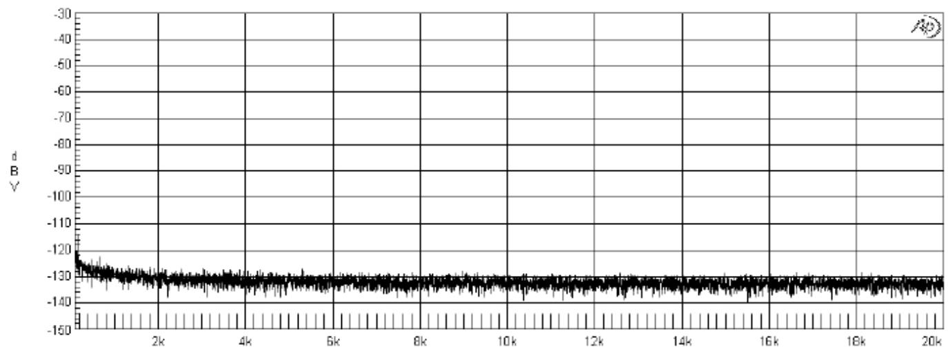
噪音测试：Vdd = 5.0V , Gain = 20dB, BW<22kHz
